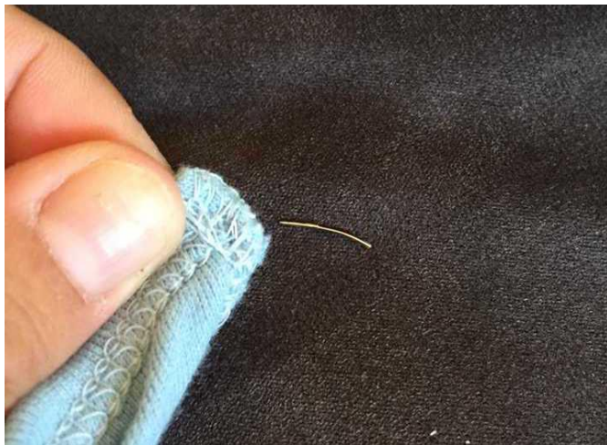
Broken point of machine needle found in underarm seam of infants bodysuit (May)
