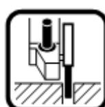
When cutting, do not press, tilt or oscillate. Gently slide it forward with a speed adapted to the material being worked on.
