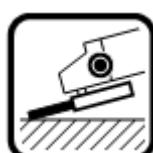
The best roughing results can be achieved with a 30°-40°approach angle. Move the machine back and forth with moderate pressure. In this manner, the work piece will not overly heat up or discolor and no ridges will be formed.
