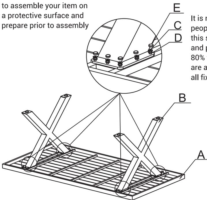
It is recommended that 2 people are required on this step, Install all fixings and parts into location and 80% tighten, once all parts are aligned 100% tighten all fixings
