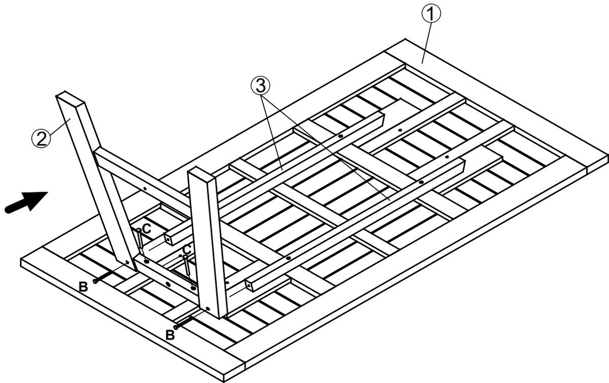
STEP 3: Attach assembled frame from step 1 to assembled frame from step 3. Insert screw (B) through leg frame (2) into brace rail (4). Tighten with allen key (E).
