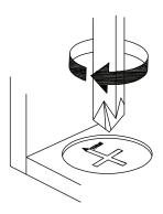
Turn cam lock clockwise to tighten.
