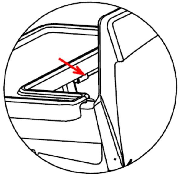
**WARNING:** Always ensure the tray is locked correctly before use.
