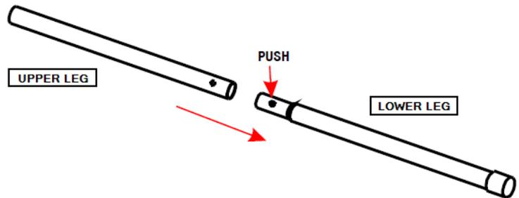
Once assembled, attach legs to the chair body, taking care that front and back legs are in the correct location. Ensure that the button clicks through the corresponding hole in each case.
