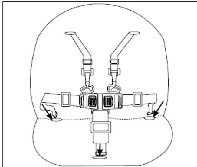
Ensure the waist straps and crotch strap are fed through the slots in the seat cover and are correctly fitted to the chair frame.
