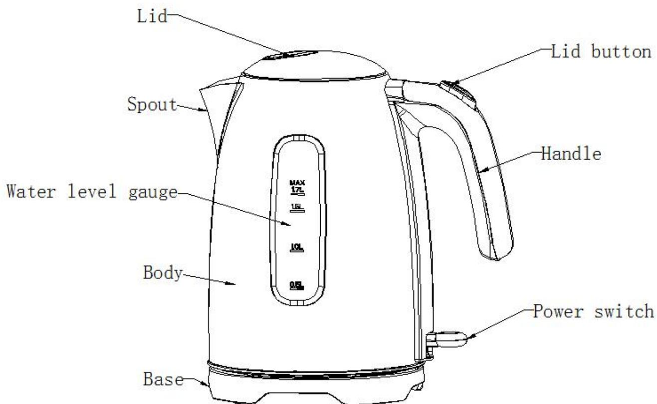
Note: Spout filter is located on the inside, accessible after opening the lid.
