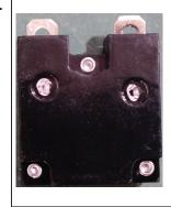
The internal circuit breaker (fitted inline with the battery) will cut off the power if the ride on is overloaded. Once the overload has been removed, the device will automatically reset within seconds.
