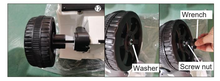
12. Insert the driving wheel to the motor side and another rear wheel to the washer side, add one washer to each rear wheel, then screw nut and use wrench to tighten the wheel.
